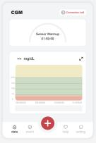
Tap"Start" to begin 2-hour sensor warm-up. There will not be any glucose readings or alerts until warm-up has ended. Keep the App open and your smart device within 20 feet of the transmitter during the sensor warm-up.
